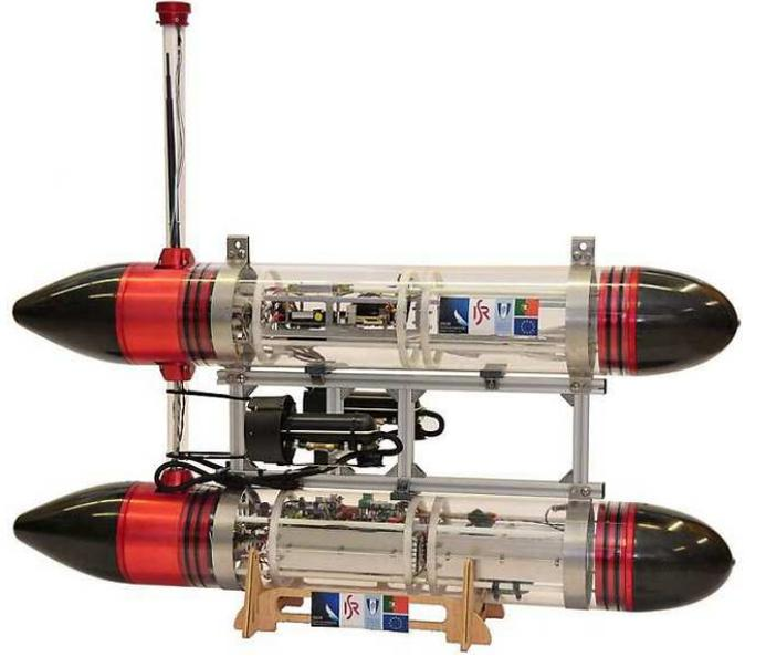
Fig. 2. The MEDUSA<sub>s</sub> surface craft. The thrusters are mounted in the middle between both hull parts on the  $x$ - $z$ -plane (body coordinates) and produce completely from the body on the  $x$ - $y$ -plane.
