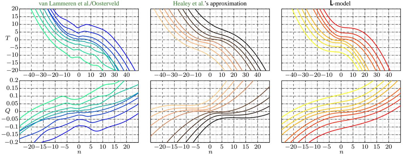
Fig. 2. Level curves of four-quadrant thrust  $T$  and torque  $Q$  as obtained from the original data published by Oosterveld, the approximation of Healey et al., and the L-model. The plots show thrust and torque for different values of the advance velocity ( $v_a \in [-2, 2] \frac{m}{c}$  with a step size of  $0.5 \frac{m}{c}$ ; darker colors are negative, lighter colors are positive  $v_a$ ).
