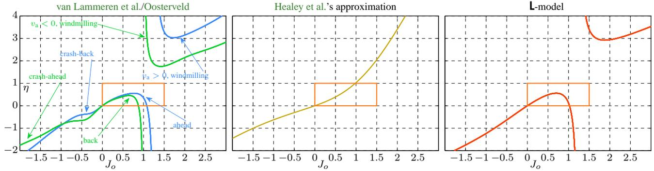
Fig. 5. Comparison of the open-water efficiency  $\eta(J_0)$  for the different propeller models, computed for  $v_a \in \{-2.0, -1.5, -1.0, -0.5, 0.0, 0.5, 1.0, 1.5, 2.0\} \frac{\text{m}}{\text{s}}$  and  $v_p$  such that the full range of  $360^\circ$  for  $\beta$  was covered for each value of  $v_a$ .
