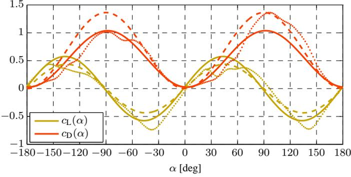
Fig. 4. Lift and drag coefficients. The figure shows the original Fourier series data (the **O**-model, dotted), the **H**-model (dashed), and the **L**-model (solid).
