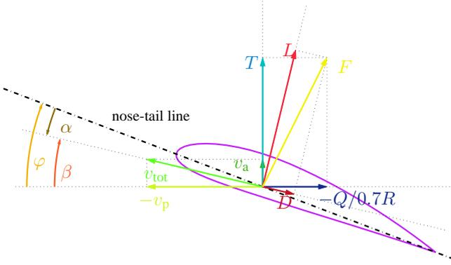
Fig. 1. Forces and velocities acting on a propeller blade. The propeller is assumed to be left-rotating for forward-thrust generation, i.e. the vehicle (and thus the propeller) is moving upwards in this picture, while the propeller to the left (i.e. into the page).
