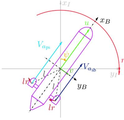
Fig. 2. Conceptual drawing of the MEDUSA as seen from above. The arrows illustrate the velocities experienced at different points of the body for a system that is undergoing a right turn with  $r = 0.1\text{s}^{-1}$  while moving forward with  $u = 1.0\text{ms}^{-1}$ . The black coordinate axes represent the body frame  $\{B\}$ , the grey axes the inertial frame  $\{I\}$ .
